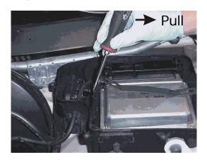
Remove the sprung bracket that holds the ECM in place by gently prying with a flat-head screwdriver as shown in the photograph.
