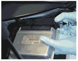
Next, remove the two electrical plugs attached to the rear of the ECM. This can be accomplished by pulling the release mechanisms on each plug (see photo).
