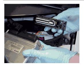
Attach electrical plugs to the ECM ensuring that the plugs are fully seated and release mechanisms are pushed all the way in. Snap sprung bracket back into place on top of ECM. Check that ECM is properly positioned in case.
