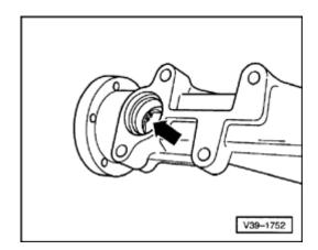
Open out circlip (arrow) on drive flange and push circlip toward splines.
