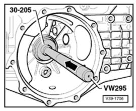
Fig. 10 Driving outer race for small tapered roller bearing into transmission housing
