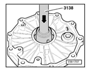
Fig. 11 Driving outer race for large tapered roller bearing out of cover
