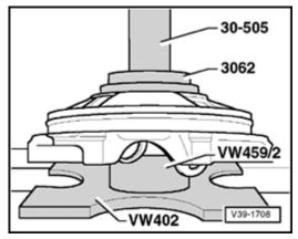
Fig. 12 Driving outer race for large tapered roller bearing into cover
