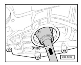
Fig. 9 Driving outer race for small tapered roller bearing out of transmission housing
