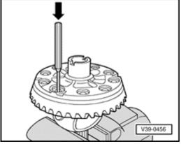
Fig. 5 Driving ring gear off housing
