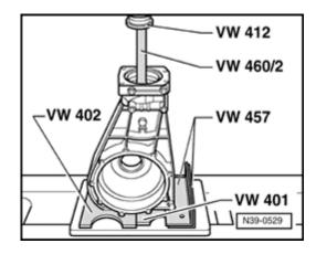
Fig. 3 Pressing drive pinion out of inner race for small tapered roller bearing
