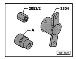
Fig. 1 Tools for loosening and tightening drive pinion nut
