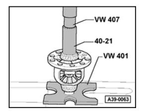
Fig. 6 Pressing on inner race for large tapered roller bearing
