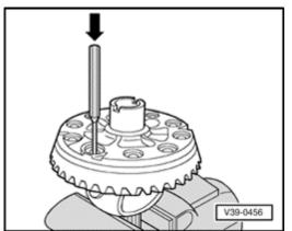
Fig. 9 Driving ring gear off housing
