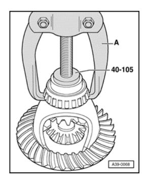
Fig. 3 Pulling off inner race for small tapered roller bearing
