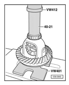
Fig. 4 Pressing on inner race for small tapered roller bearing
