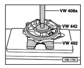
Fig. 8 Pressing outer race for large tapered roller bearing into cover
