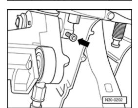
✓ Do not tighten bolt (arrow) until both securing clips have been fitted on the clutch pedal/brake pedal pivot pin.
