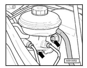
Tighten bolts for brake booster (arrows) to 25 Nm.
