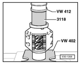
Fig. 2 Pressing on ball bearing for Torsen differential
