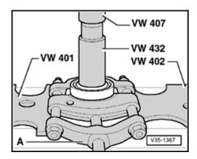
Fig. 1 Pressing off ball bearing for Torsen differential
