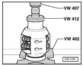
Fig. 4 Pressing on inner race for needle bearing for Torsen differential
