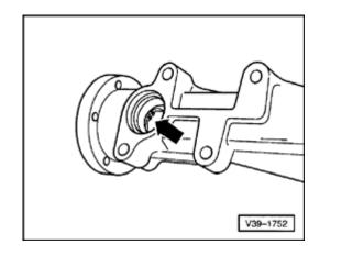
Expand circlip (arrow) on drive flange and slide in direction of notched splining.
