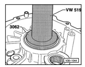
Install double tapered roller bearing outer race for pinion shaft in transmission housing without shims ⇒ Fig. 3, Page 35-31.
