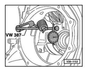
Rotate pinion shaft together with hollow shaft 5 turns in each direction to settle tapered roller bearing. Otherwise measurement will not be correct.
