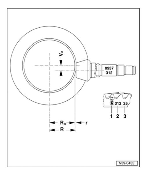
Adjustment and marking of final drive gear sets
