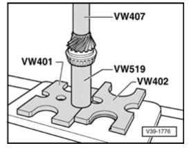
Fig. 7 Installing large tapered roller bearing inner race onto pinion shaft
