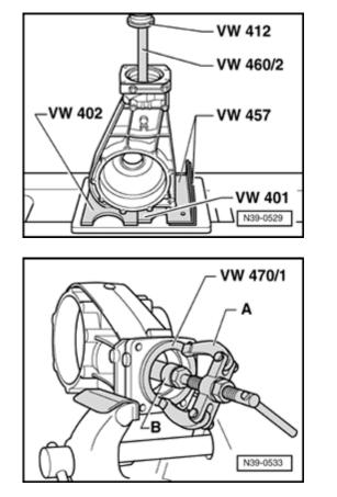
Fig. 3 Removing pinion shaft from small tapered roller bearing inner race
