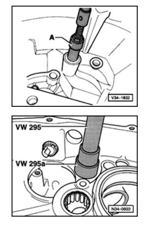
Fig. 3 Removing bushing for 3rd and 4th gear shift rod
