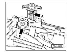
**<** Installation position of complete gear lock in transmission:
