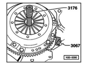
Fig. 1 Centering clutch plate and removing and installing pressure plate
