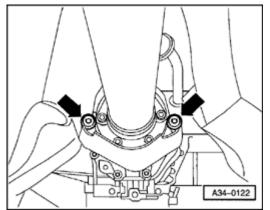
Unbolt heat shield for driveshaft from cover for Torsen differential (arrows).
