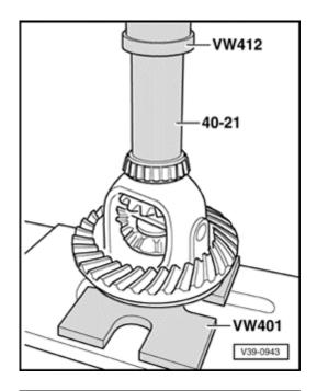
Fig. 4 Pressing on small tapered roller bearing inner race
