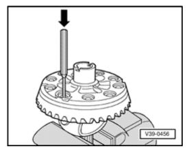
Fig. 9 Driving out ring gear from housing
