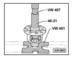
Fig. 6 Pressing on large tapered roller bearing inner race
