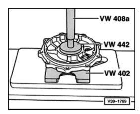
Fig. 8 Pressing large tapered roller bearing outer race into cover
