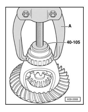
Fig. 3 Pulling off small tapered roller bearing inner race
