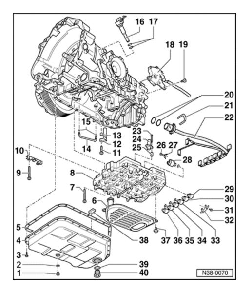
Overview of the removed parts for transmission with Park/Neutral Position (PNP) Switch -E17-
