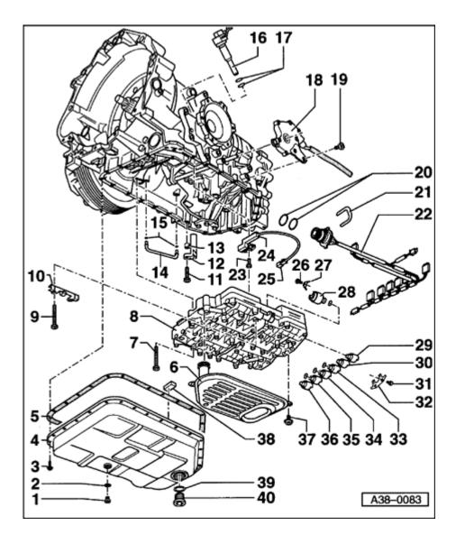
Overview of the removed parts for transmission with hydraulic control E18/2
