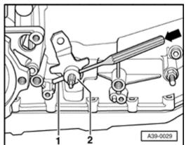
Drive out spring dowel sleeve -1- at lever/shift rod -2- in direction of travel toward the front (arrow), until the lever/shift rod can be pulled off the shift rod.
