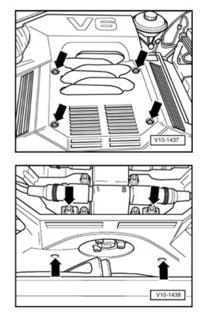
Fig. 1 Unclipping and removing top engine cover
