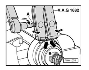
force required on the clamp will not be achieved even though the correct tightening torque is indicated.
