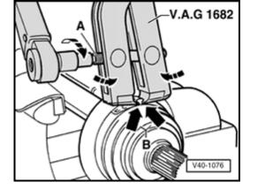
Clamps used on rubber joint boots are tightened using VAG1275 pliers
