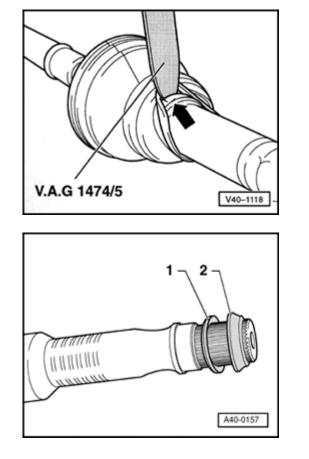
Fig. 4 Positioning boot over bead of profiled shaft
