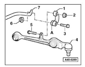
Bonded rubber bushings can only be turned a limited amount. Therefore only tighten bolted connections at the suspension links when the vehicle is standing on the ground.
