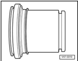
Fig. 3 Installing the outer sealing lip of the protective seal onto the piston
