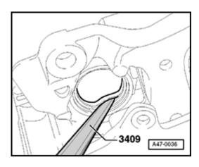
Fig. 2 Removing seals using 3409 wedge
