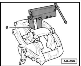
Fig. 5 Pressing piston into brake caliper housing using piston resetting tool
