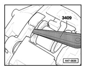
Fig. 4 Installing inner sealing lip of protective seal using 3409 wedge
