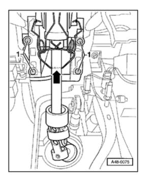
Secure steering column with safety wire before removing steering column from steering gear pinion.
