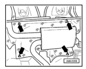
Remove heat shield (arrows) at rear muffler and push to side.
