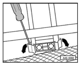
Open cable clamp (arrows) and remove parking brake cables.
