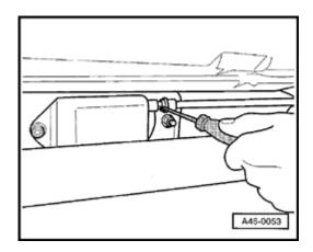
Use screwdriver to pry parking brake cable out of bracket.
