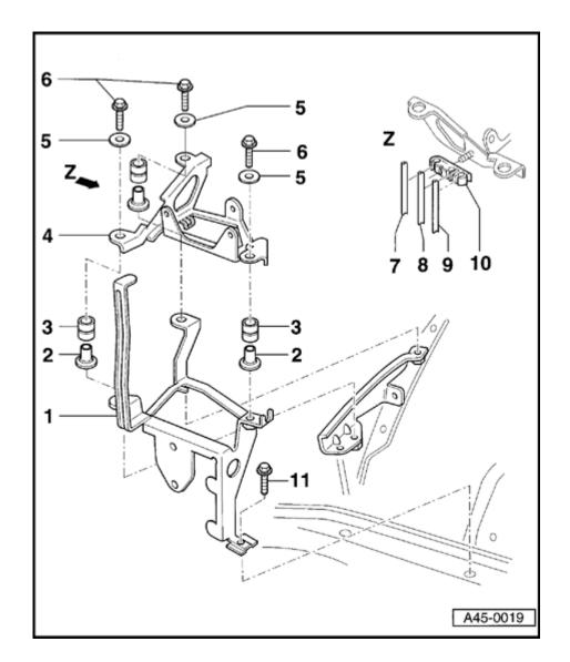
ABS hydraulic unit mounting bracket, removing and installing
