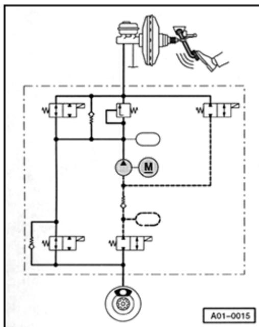
▲ The hydraulic circuit diagram shows a systematic representation of an ABS/EDL system. This will give a better understanding of the various test steps in the output Diagnostic Test Mode (DTM).
