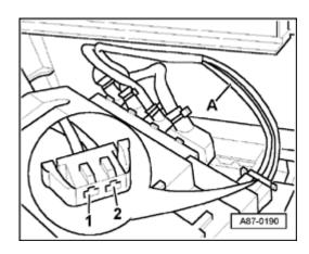
Disconnect harness connector E from A/C control head -E87-.
