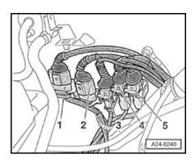
Connect VAG1598/31 test box at wiring harness to Engine Control Module (ECM), do not connect ECM ⇒ Page 24-19.
