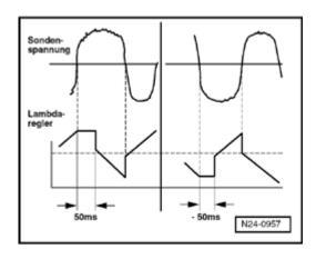
It corrects slight changes in the mixture (i.e. enrichment) via the oxygen sensor before catalytic converter by holding oxygen sensor control before catalytic converter at its higher or lower point for a specific time (dwell time). If this time is in the positive range (i.e. 50 ms), mixture is shifted in the -enrich- direction. If it is in the negative range (e.g. -50 ms), mixture will be shifted in the -lean- direction.
