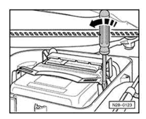
Using a screwdriver, carefully pry off retaining bracket (arrow).
