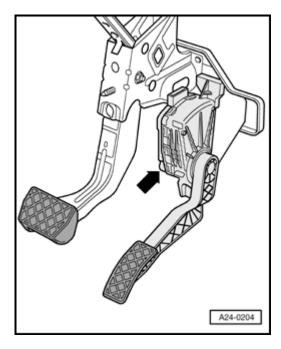
Fig. 5 Installation position, Throttle Position (TP) sensor -G79-and sender 2 for accelerator pedal position -G185-
