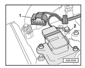
Disconnect 4-pin harness connector -1- at ignition coil -2-.
