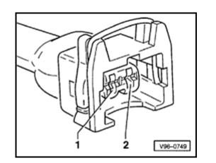
Check wiring for continuity between intake manifold change-over valve harness connector terminal 1 and fuse, using wiring diagram.
