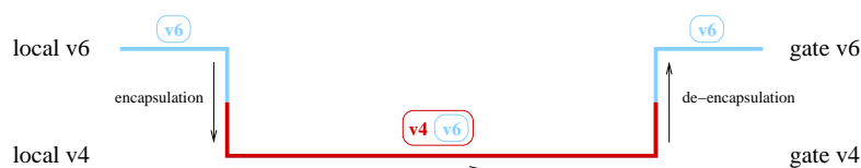
Figure 8-7. A frequently used method for transition is tunneling IPv6 in IPv4 packets
