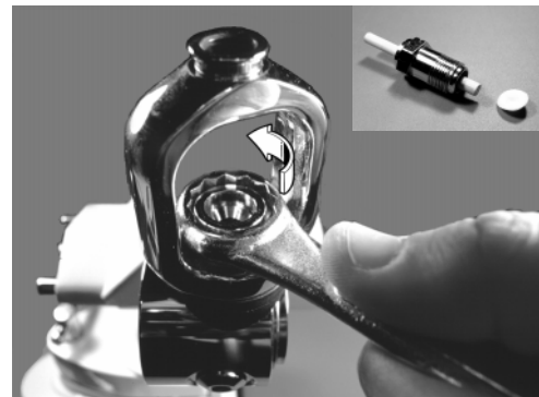
Figure 6 Removing Yoke Connector
