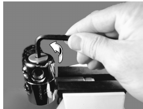
Figure 5 Removing Turret Retaining Bolt
