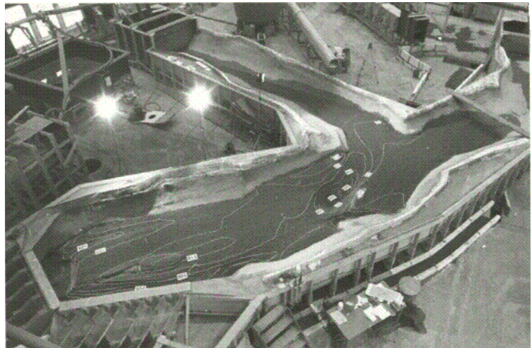
Fig. 9.9.1 Photo of the physical model made at SINTEF, Norway, for the Kali Gandaki hydropower plant in Nepal. The model was used to investigate sediment flushing from the hydropower reservoir. The dams are shown in the lower left corner. The water is fed into the model at the upper left part of the picture. The model is approximately ten meters long from the dam to the end shown on the right. The model was built of concrete according to the prototype bed, and filled with sand to the level of the spillway crest. The model was then carefully filled with water, and then the flushing started by opening the dam gates. As the run-of-the-river reservoir is fairly narrow, much of the sediments was removed by the flushing
