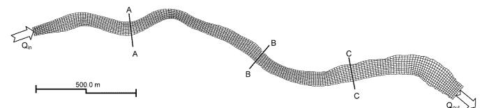
Figure 3: Grid for the flushing simulation with 15,358 cells and the cross sections A - C
