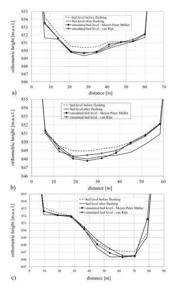
Figure 4: Bed level changes, measured and simulated with van Rijn and Meyer-Peter Müller bed-load transport formulas
