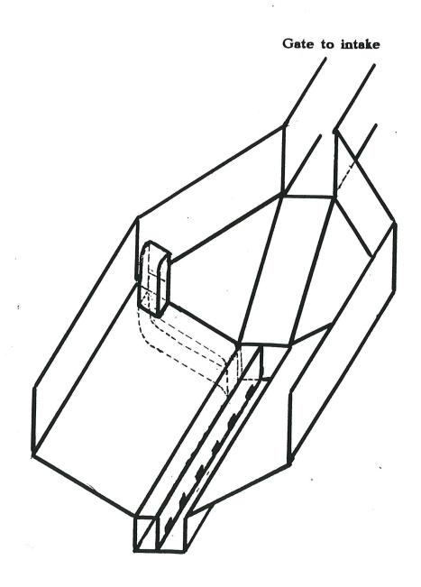
An important point is to try to minimize the head loss through the entrance. Therefore, it should be designed with a large cross-section and all the bends should be hydraulically well shaped to give as small loss as possible.
