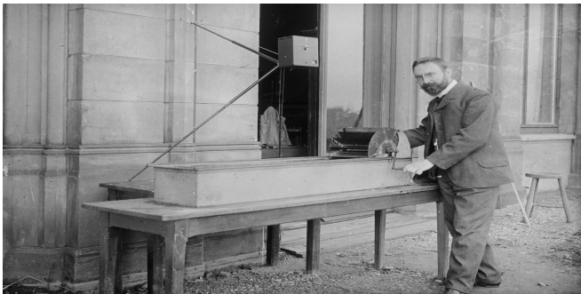
Ludwig Prandtl in front of his water tunnel for flow visualization in 1904.
