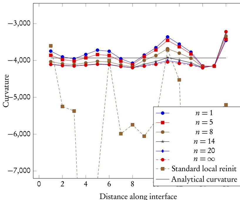
Figure 4.4: Lineplots of curvature along the interface for different exponent  $n$  in the geometric weighting.
