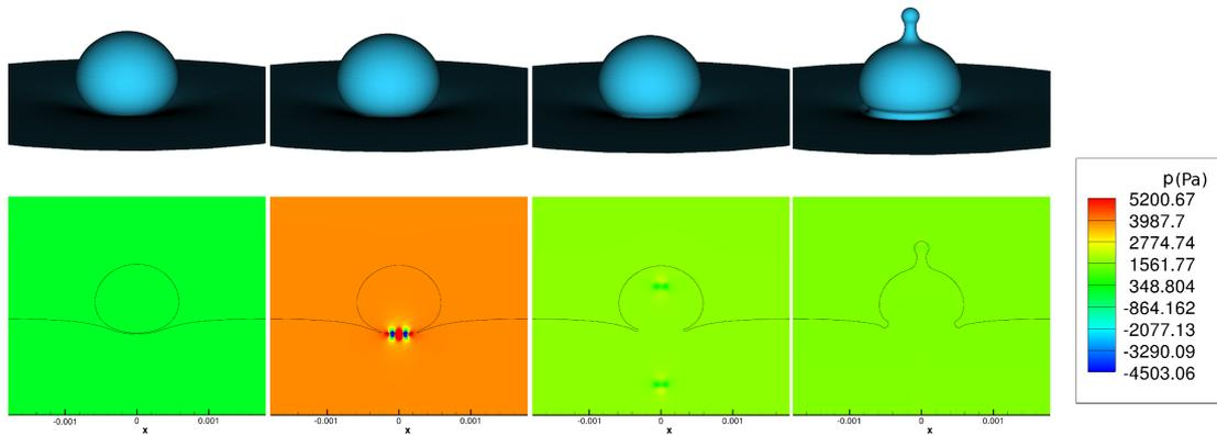
Figure 5.18: A droplet merging into a pool produces an unphysical pressure wave, causing the top of the droplet to jet upwards. The pressure field is shown in the lower half of the figure, where a wave originating at the time of merging can be seen.
