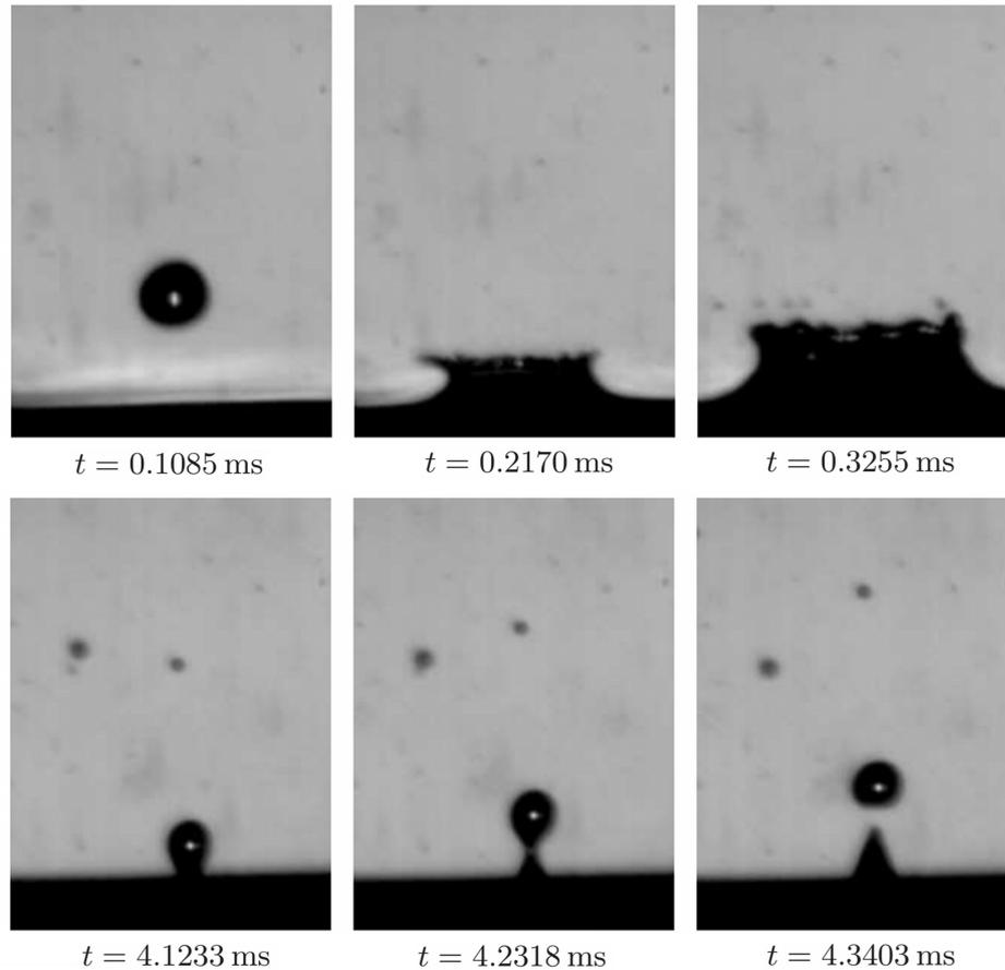
Figure 6.3: High-speed imagery of a 0.26 mm diameter n-pentane droplet impacting a pool of n-pentane at 5.9 m/s. After some time, the surface of the pool rebounds and ejects a jet. Note that some time has passed between the first and the second row of images. Figure from [52, Figure 5.6].
