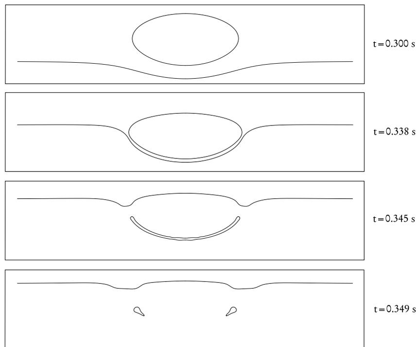
Figure 5.19: Attempt at simulating the droplet-pool case studied by Mohamed-Kassim and Longmire. In this case, the droplet is ten times larger than in the previous simulations reported. This simulation does not agree with experiments, as the merging here happens much earlier than in experiments.
