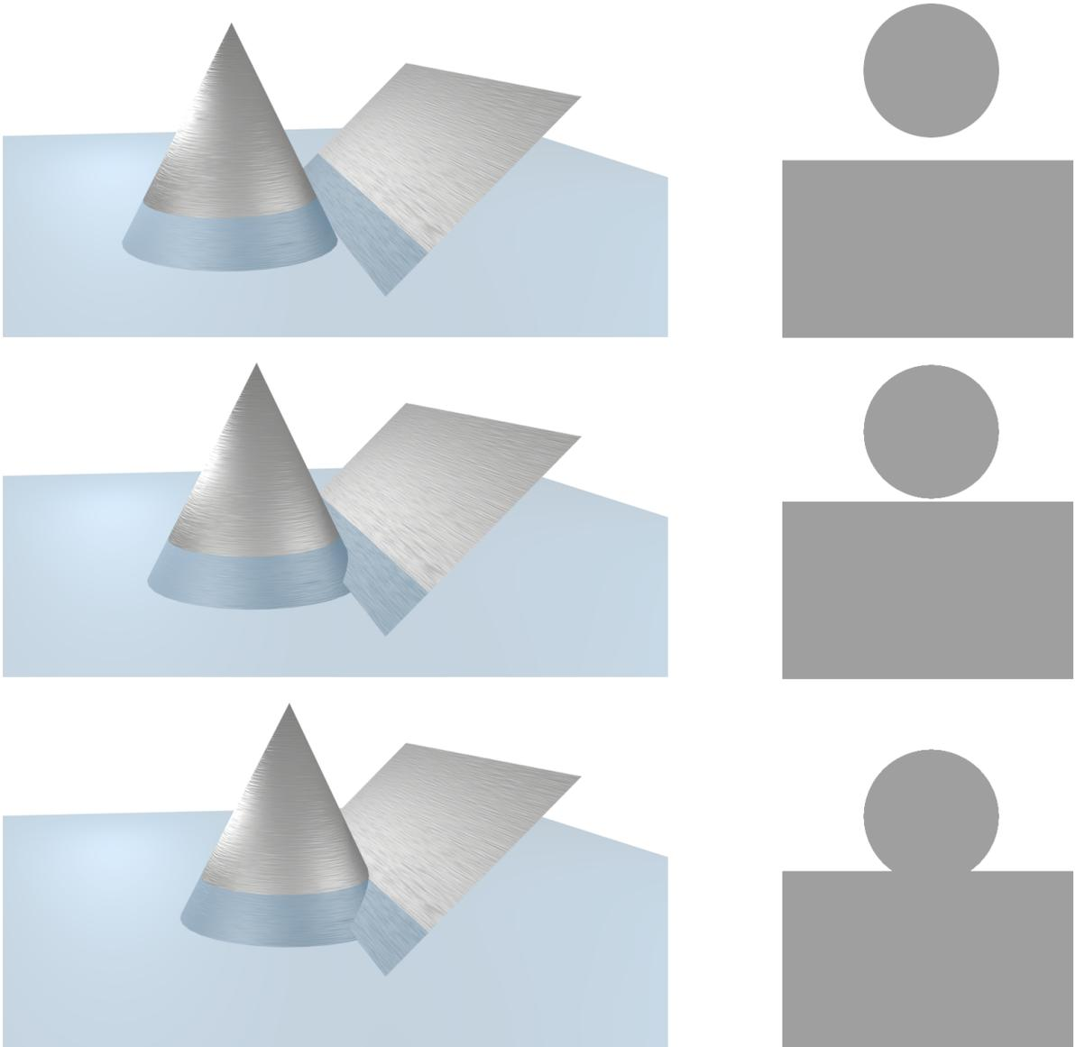
Figure 1.1: Illustration of interface tracking using the level-set method. The interface is between the grey and the white area on the right-hand side of the image, and the level-set function is shown in grey on the left-hand side. Also shown on the left-hand side, in blue, is the plane  $\phi(\mathbf{x}) = 0$ .
