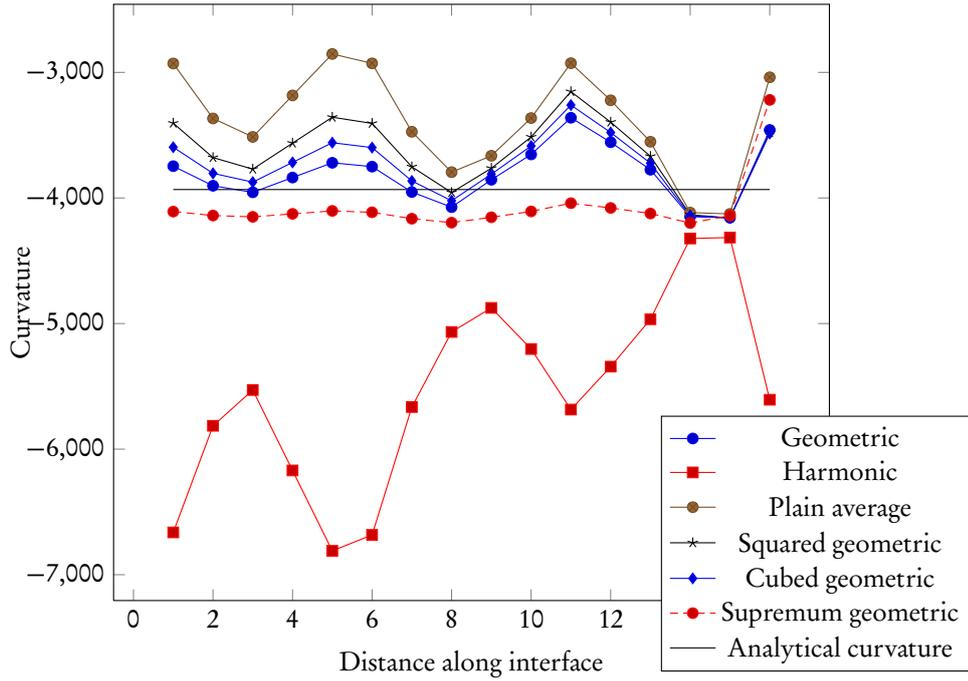
Figure 4.3: Lineplots of curvature along the interface for different averaging methods.
