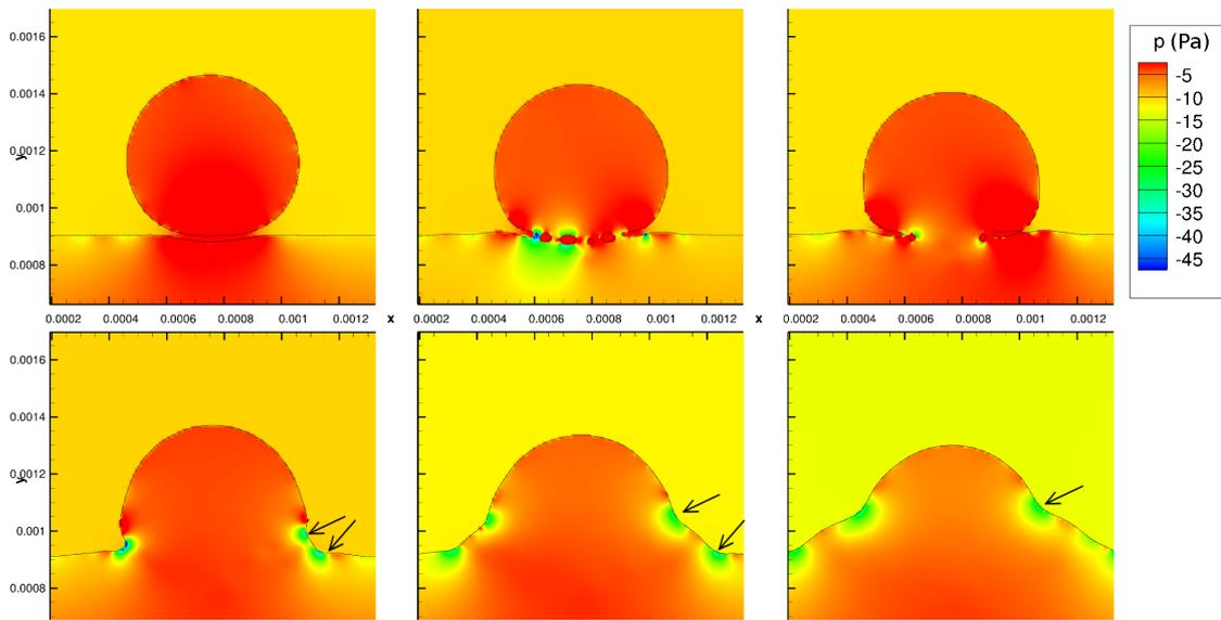
Figure 5.8: Methanol droplet merging with pool of methanol. The pressure field is indicated in color. There are still pressure instabilities, as can be seen, but not as bad as in previous cases. Apart from the problematic pressure, the merging is seen to progress reasonably, with two capillary waves seen on each side (indicated in arrows on the right side). The snapshots are 3 ms apart.
