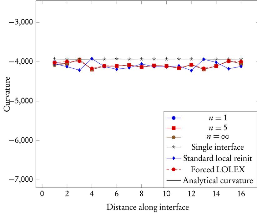
Figure 4.5: Lineplots of curvature along the interface using different averages, when the distance between interfaces is  $2.2\Delta x$ . Here it is seen that the difference between the averages is much smaller than for the previous line plots.
