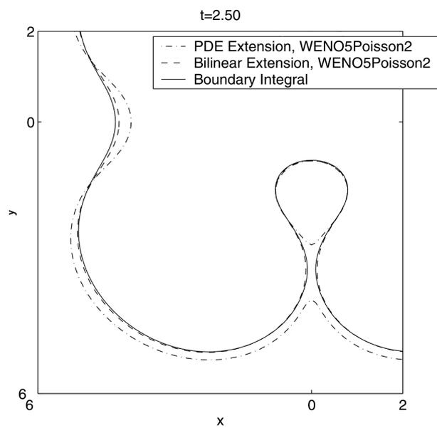
Figure 3.4: Another typical situation where the Salac and Lu method would fail. Figure copied from [24], showing the interface between a tumor and healthy tissue. The dash-dotted line is the least accurate solution.
