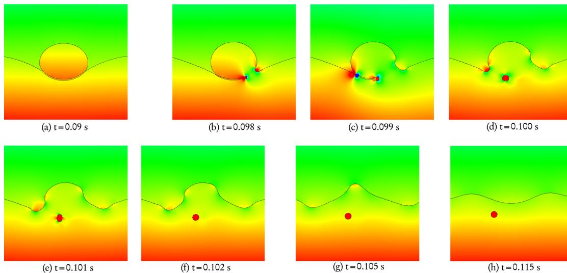
Figure 5.11: The behaviour during and after merging for the water-in-decane case in 2D, using the fine ( $350 \times 390$ ) grid. The times are indicated below each frame. The pressure field is indicated in color, and is stable and looks sensible. Note that increased spacing between frames indicates that a longer time interval has passed between these frames.
