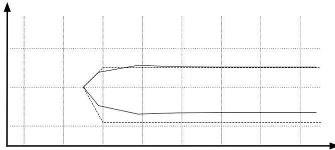
Figure 4.8: Thin body deformed by reinitialization. The dotted line shows the initial interface, where  $\phi$  is a signed distance function. The full line shows the result of reinitialization. In theory these should overlap. The width of the initial body is  $1.45\Delta x$ .
