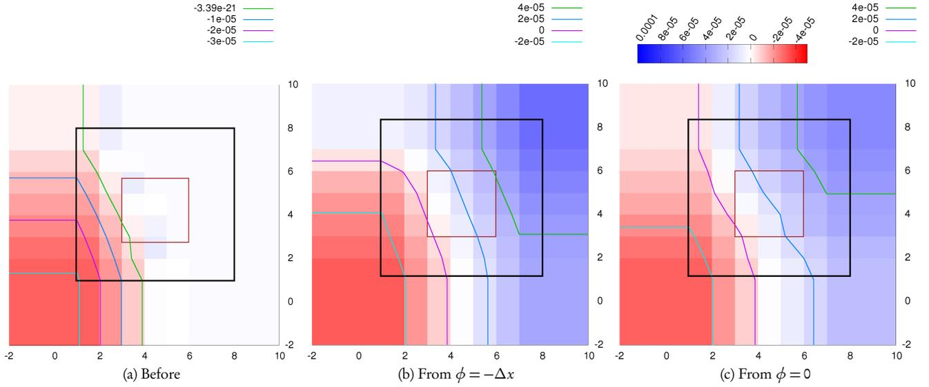
Figure 3.10: The LOLEX method on a global level set which is distorted due to reinitialization of very close bodies. (a) Local  $\phi$  before reinitialization. (b) Local  $\phi$  reinitialized from  $\phi = -0.8\Delta x$ . (c) Local  $\phi$  reinitialized from  $\phi = 0.0$ . The black square indicates the boundary to the ghost cells, and the red square indicates the  $3 \times 3$  central points that are used in the final curvature calculation.
