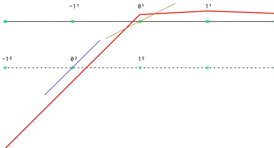
Figure 3.9: Why we reinitialize from a lower level set: At the lower level set, indicated by the dotted line, values of e.g.  $\nabla\phi$  are more accurate at the grid point which is closest to the red line than for the zero level set. The red line indicates the local level-set function  $\phi$ .
