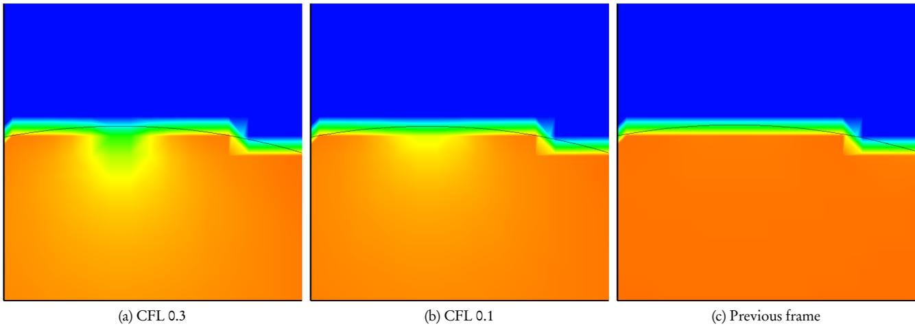
Figure 5.7: Effect on stability of reducing the CFL number. The CFL number is reduced from 0.3 to 0.1, which reduces the instability somewhat, but does not remove it. The frame after the one in (a) and (b) is shown in (c); here, no trace of the instability is seen. The frame prior to (a) and (b) is identical to (c) with regards to the pressure.
