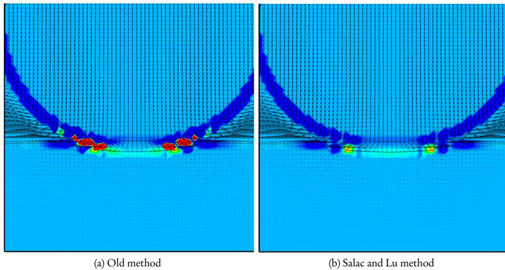
Figure 5.2: Why the ordinary method fails: the curvature field is plotted in the last frame before the crash, for the old method and for the Salac and Lu method (which does not crash in its next frame). The light blue background indicates zero curvature, the dark blue indicates a negative value, and red indicates a positive value. The curvature calculated by the Salac and Lu method is correct.
