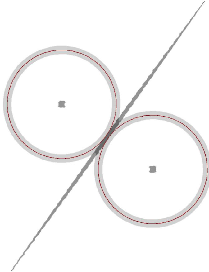
Figure 3.5: Illustration of the quality function and the narrow band level-set method. The red lines indicate  $\phi = 0$ , the light grey bands indicate the narrow band where  $|\phi| < \epsilon$ , and the medium grey band indicates where  $Q(\mathbf{x}) > \eta$ . The intersection of the light and the medium grey bands, the dark grey area, indicates where the LOLEX method will be used.
