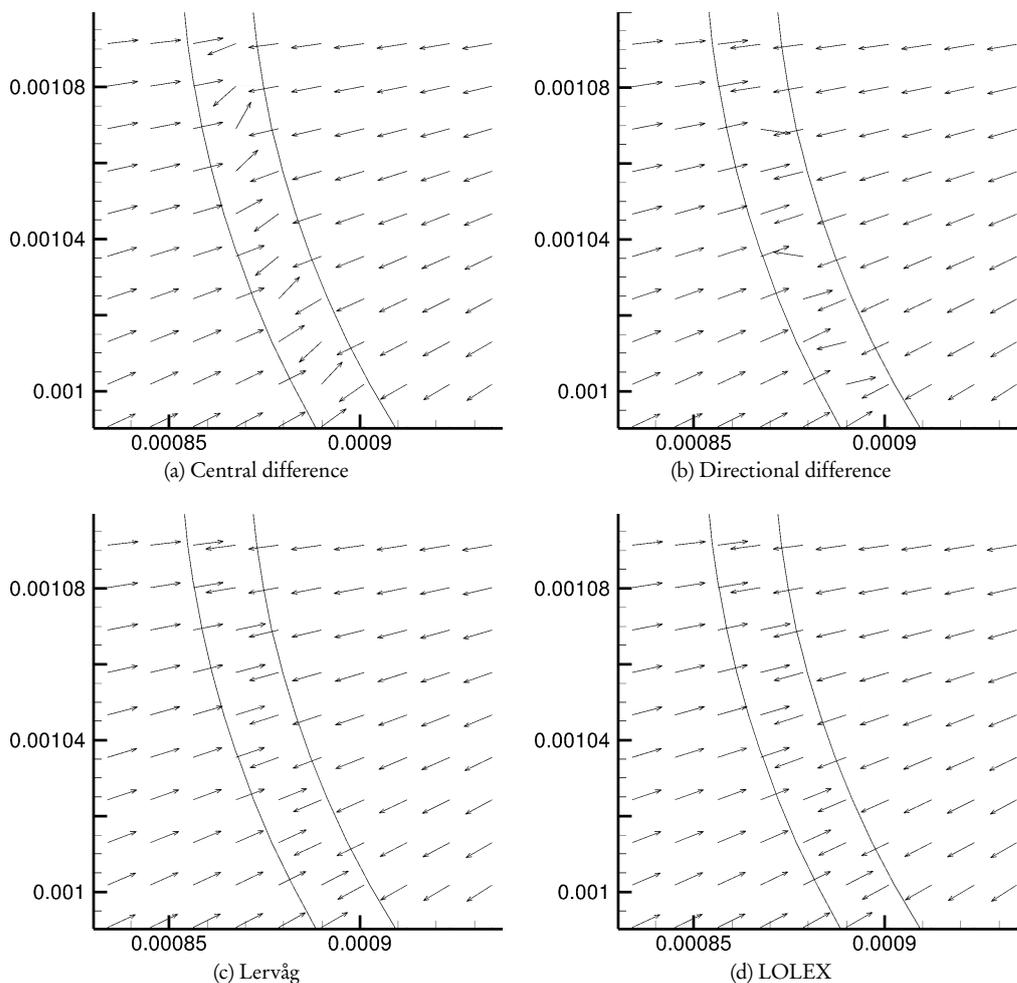
Figure 4.9: Comparison of normal vector calculations using different methods.
