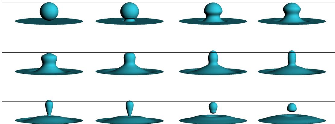
Figure 5.16: Axisymmetric simulation of a water droplet immersed in a decane-polybutene mix, merging with a deep pool of water. The capillary waves travelling up the bubble after merging are clearly seen. After some time, pinch-off occurs, and a new droplet is formed. The black lines indicate the top of the droplet just before merging.
