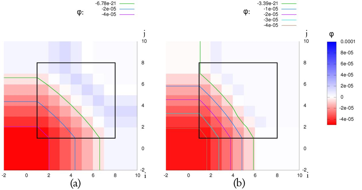
Figure 3.8: Zeroth-order extrapolated local level set, part of a circle. In this case, there are 7 internal cells in either direction, and three ghost cells outside this. The black square frames the internal cells. In (a), the distance from the interface to the other body is  $2.8\Delta x$ . In (b), the distance is  $1.1\Delta x$ . It is seen that the zero level set in (b) is slightly deformed.
