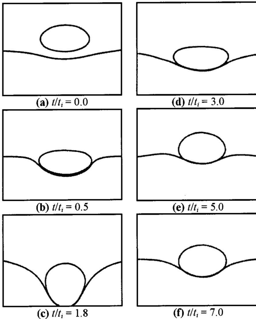
Figure 6.7: Snapshots of a droplet of water and glycerin falling through a mineral oil, and then colliding with a pool. The droplet deforms the pool significantly, before the pool bounces back up again. The droplet does not merge with the pool. Figure taken from [29].
