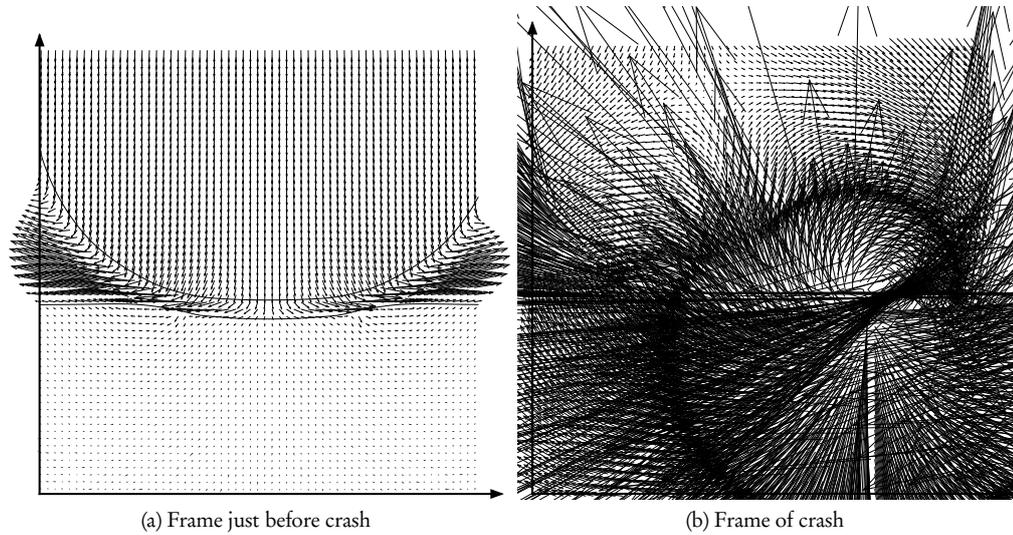
Figure 5.1: The droplet colliding with the pool, showing when the standard method crashes. The distance from the droplet to the pool is  $2.6 \Delta x$  in these figures. The velocity field is plotted, and is seen to diverge spectacularly in Figure b). The same scale is used for the vector arrows in both plots.
