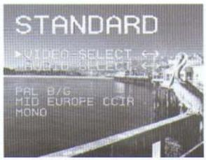
Press the rotary/pushbutton again to switch to the adjustment mode. An arrow , will appear in place of the scrolling symbol, the entry will appear in pink.
