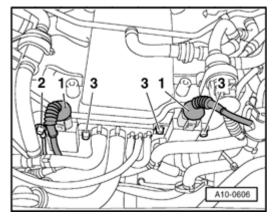
For vehicles with manual transmission, the control modules for exhaust gas temperature are at rear of intake manifold, on left and right.
