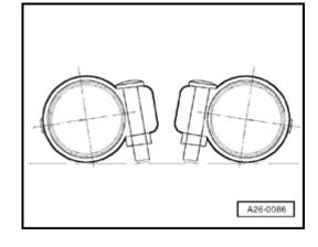
The ends of the bolts must not project below the bottom of the clamp.
